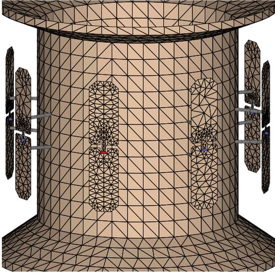
Fig. 1. UCA composed of  $N$  antenna elements in front of a cone-shaped reflector.
