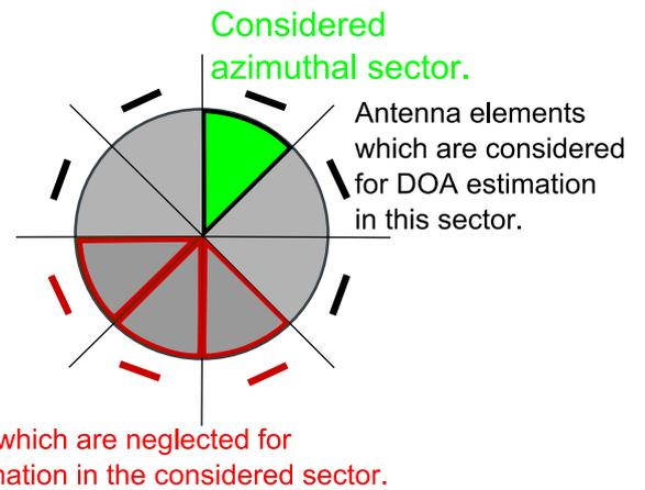
Fig. 4. Example for the allocation of antenna elements in front of a cone shaped reflector to a sector.
