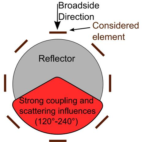
Fig. 2. Azimuthal range with good receiving properties for one element in front of a cone shaped reflector.
