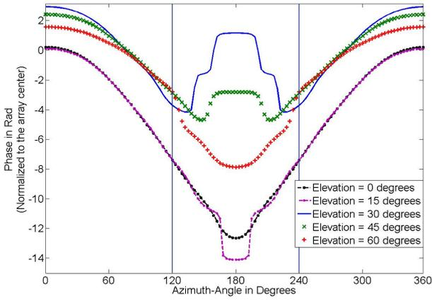
(a) Phase of the receiving characteristic of one UCA element in front of a cone shaped reflector.
