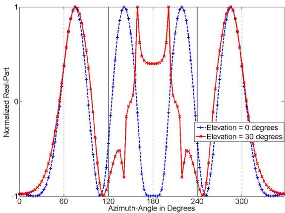
(b) Real part of the receiving characteristic of one UCA element in front of a cone shaped reflector.
