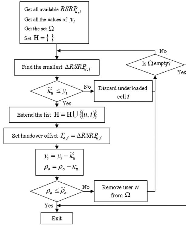
Fig. 1: The selection process of the candidate UEs that is followed by an overloaded cell.
