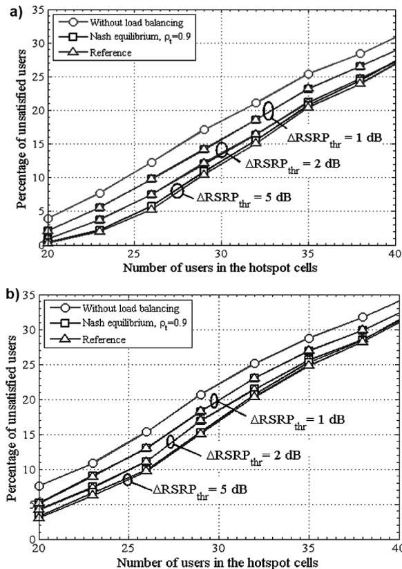
Fig. 5: Performance of the (a) homogeneous and (b) heterogeneous networks as a function of number of users in the hotspot cells with the link imbalance threshold  $\Delta RSRP_{thr}$  as parameter.
