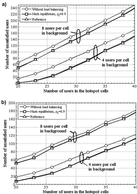
Fig. 3: Performance of the (a) homogeneous and (b) heterogeneous networks as a function of number of users in the hotspot cells with number of users per cell in background as parameter.
