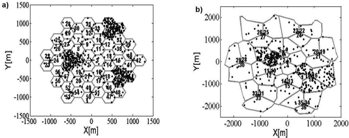
Fig. 2: (a) Homogeneous and (b) heterogeneous networks with nine and six generated hotspot cells respectively.
