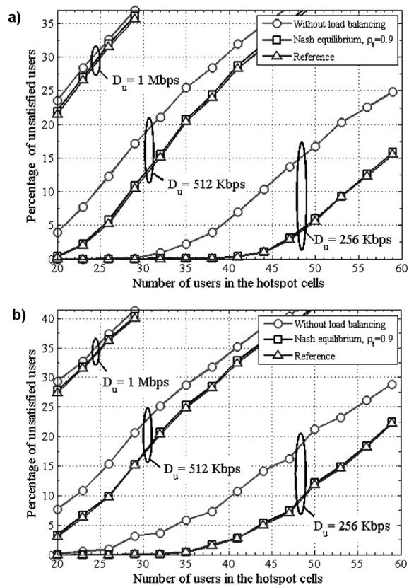
Fig. 4: Performance of the (a) homogeneous and (b) heterogeneous networks as a function of number of users in the hotspot cells with the data rate requirement  $D_u$  of the users as parameter.
