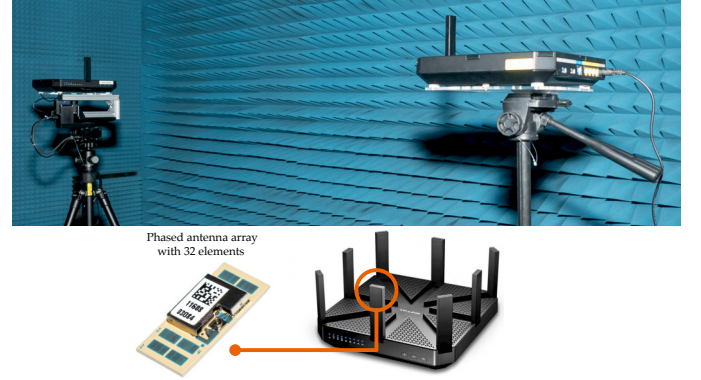
Fig. 5: The measurement setup in the anechoic chamber (top) and the close-up view of the routers and the antenna array (bottom).
