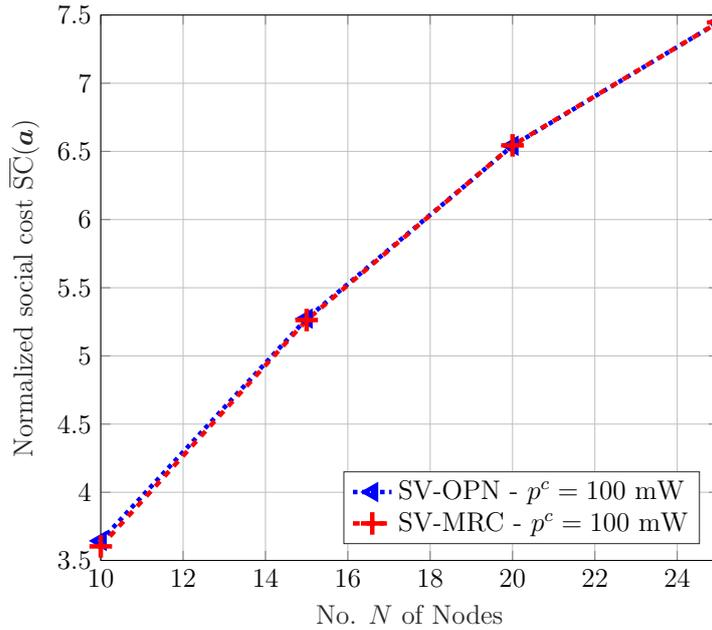
(b) The social cost with  $p^c = 100 \text{ mW}$ .Figure 5.8. The normalized social cost for different numbers  $N$  of nodes and different values  $p^c$  of circuitry power.
