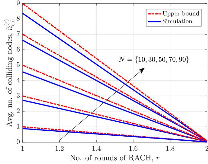
Figure 4.8. Average number of nodes that experience a collision in different rounds of RACH phases.
