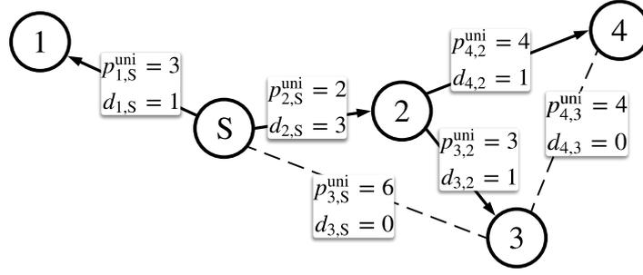
Figure 4.10. A sample BT from S to four other nodes. The numbers on the links show the required unicast powers,  $p_{i,j}^{\text{uni}}$ , and the downstream values,  $d_{i,j}$ .
