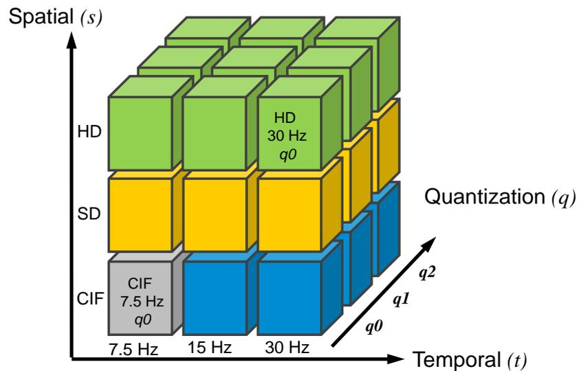
Figure 6.1. The structure of SVC coding [AZP<sup>+</sup>11]. The base layer is shown in gray.
