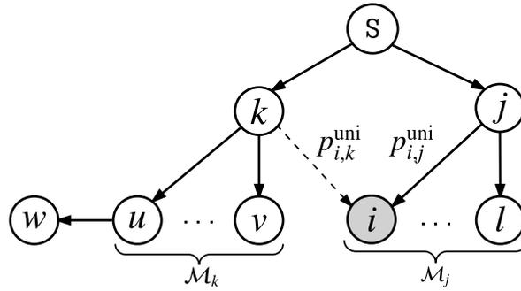
Figure 3.1. A sample network and BT. The solid arrows show the transmission from PNs to CNs and the dashed arrow represents a possible link that can be established for CN  $i$  if it chooses PN  $k$ .
