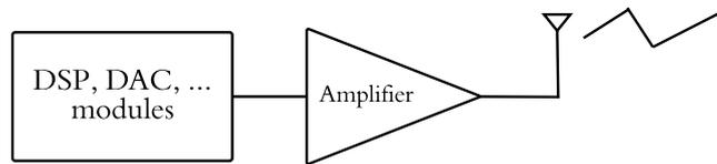
Figure 3.2. Structure of transmission modules in a transmitter.
