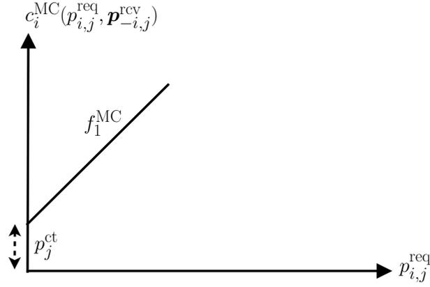
(a) The cost function of node  $i$  when  $\mathbf{1}_j(\mathcal{M}_j) = 0$ .
