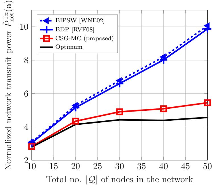
Figure 4.11. Normalized network transmit power versus the number of nodes for different algorithms.
