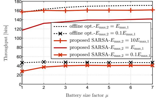
Fig. 5: Average throughput versus battery size factor  $\mu$  with  $B_{\max,l} = \mu E_{\max,l}$ ,  $E_{\max,1}/(2\sigma^2) = 5\text{dB}$ .
