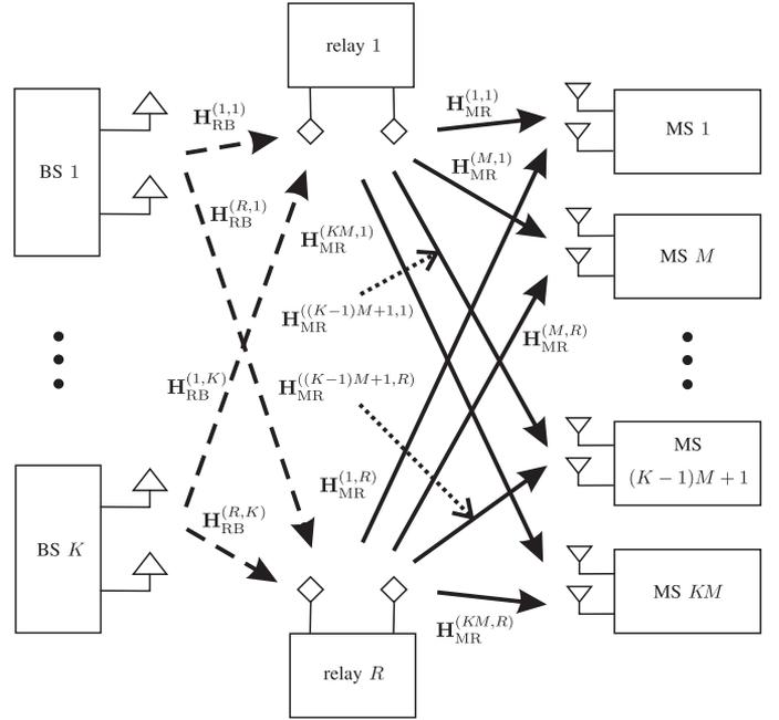
Fig. 1. A  $K$  cell scenario with  $K$  BSs,  $R$  relays and  $KM$  MSs. The transmissions in the first and the second time slot are illustrated by the dotted and solid arrows, respectively.
