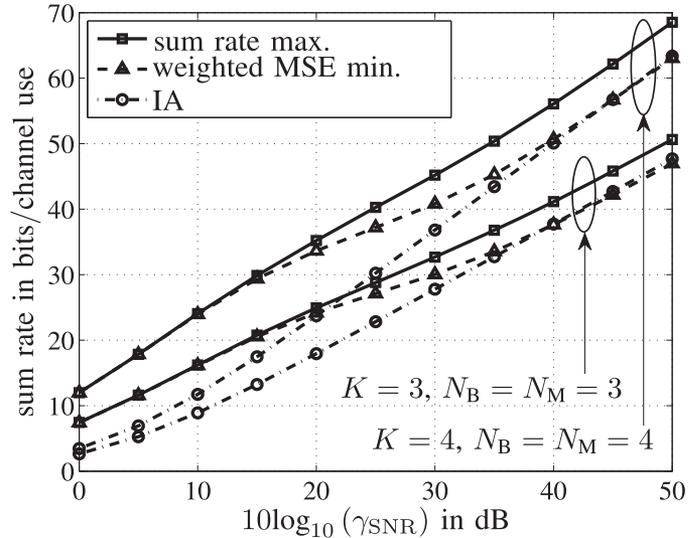
Fig. 3. Average sum rate per time slot as a function of the SNR  $\gamma_{\text{SNR}}$  in dB for scenarios with  $M = 1$  and no relays.
