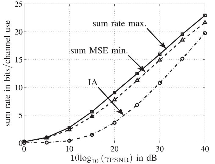
Fig. 5. Average sum rate per time slot as a function of the pseudo SNR  $\gamma_{PSNR}$  in dB for a scenario with  $K = 2$ ,  $M = N_B = 3$ ,  $R = 4$ , and  $N_R = N_M = 2$ .
