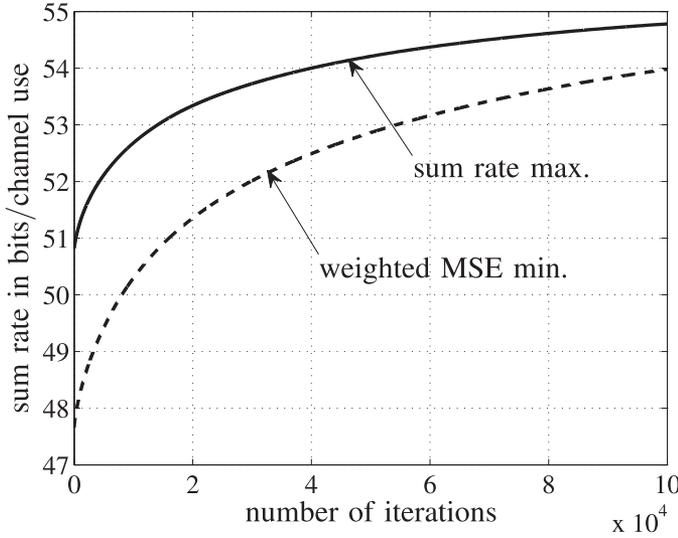
Fig. 4. Average sum rate versus the number of iterations at the SNR  $\gamma_{SNR} = 50$  dB for a scenario with  $K = 3$ ,  $M = 1$ ,  $N_B = N_M = 3$ , and no relays.
