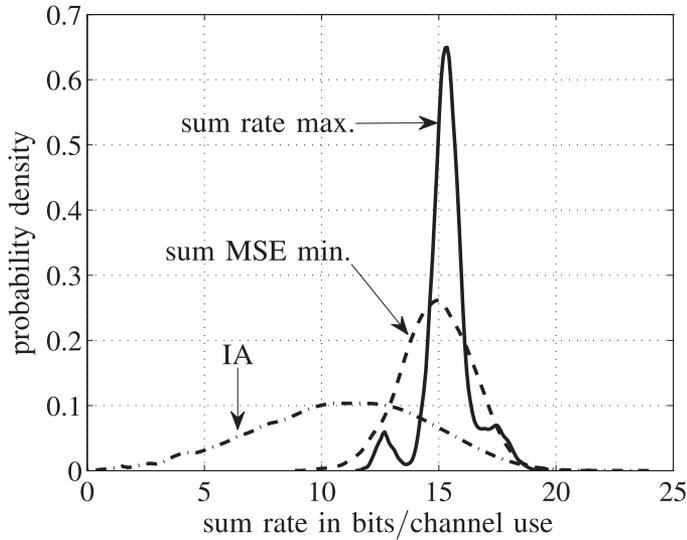
Fig. 6. Probability density of the average sum rate per time slot at the pseudo SNR  $\gamma_{\text{PSNR}} = 30$  dB for a scenario with  $K = 2$ ,  $M = N_B = 3$ ,  $R = 4$ , and  $N_R = N_M = 2$ .
