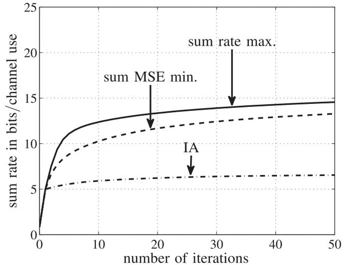
Fig. 7. Average sum rate versus the number of iterations at the pseudo SNR  $\gamma_{\text{PSNR}} = 30$  dB for a scenario with  $K = 2$ ,  $M = N_B = 3$ ,  $R = 4$ , and  $N_R = N_M = 2$ .
