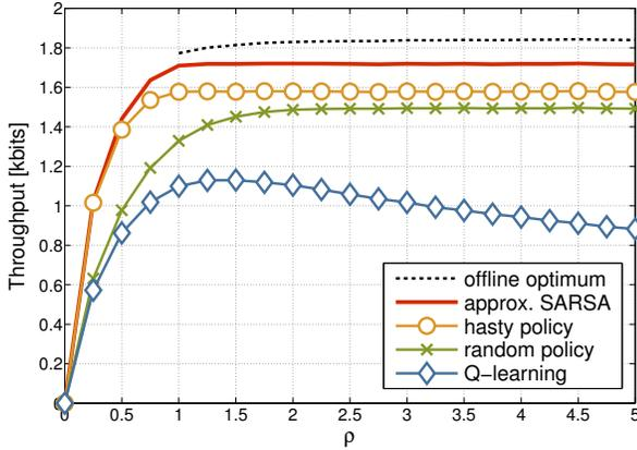
Fig. 3: Average throughput versus the battery size factor  $\rho$ . Average  $E_{\max}/(2\sigma^2) = 5\text{dB}$ .
