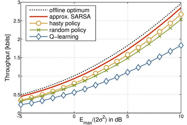
Fig. 2: Average throughput versus  $E_{\max}/(2\sigma^2)$ .
