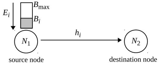
Fig. 1: Point-to-point communication scenario with an EH transmitter node.
