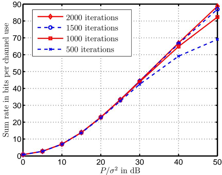
Figure 3.8. Sum rate comparison with different number of iterations for scenario B3
