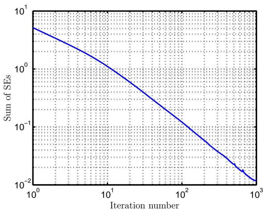
Figure 4.7. Average of the sum of SEs of different channel realizations versus the iteration number in scenario C4 with normalization of the variables
