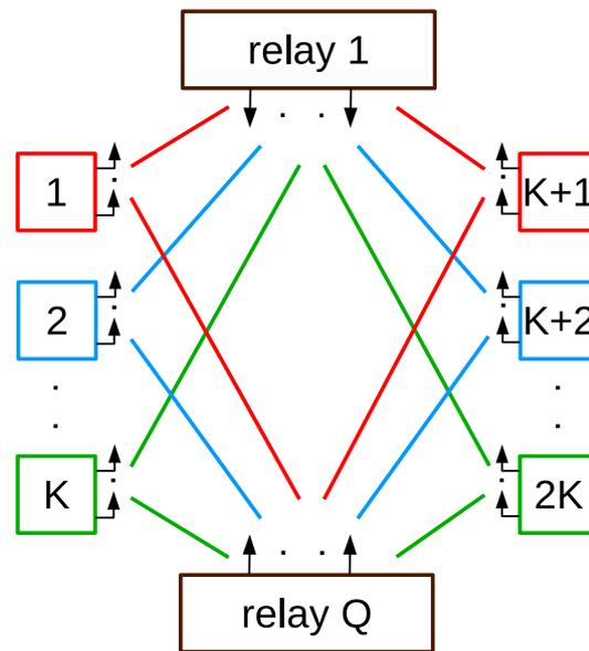
Figure 2.1.  $K$ -pair two-way relay network
