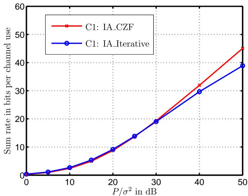
Figure 4.3. Sum rate performance of the IA\_CZF and the IA\_Iterative algorithms versus  $P/\sigma^2$  for scenario C1
