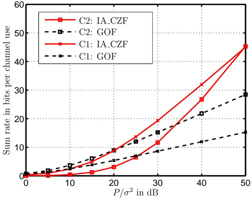
Figure 4.1. Sum rate performance of the IA\_CZF, the IA\_Iterative and the reference GOF algorithms versus  $P/\sigma^2$  for scenarios C1 and C2
