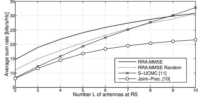
Fig. 3. Average sum rates versus different number of antennas at the RS. Scenario with  $K = 10$  nodes,  $C = 10$  subcarriers and average SNR = 15dB.
