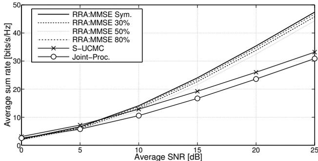
Fig. 4. Average sum rates versus average SNR at the RS. Scenario with  $K = 10$  nodes,  $C = 10$  subcarriers and  $L = 5$  antennas at the RS.
