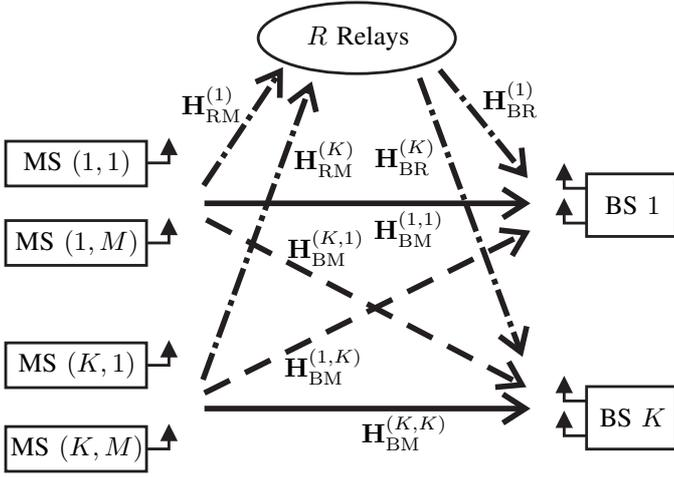
Fig. 1. UL transmission in a multicell network with multiple relays assisting the transmission
