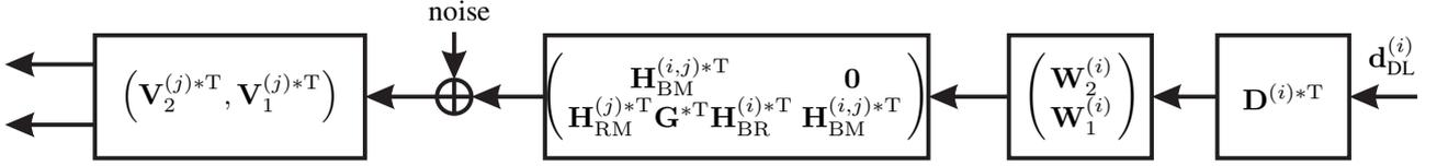
Fig. 3. Equivalent block diagram of the dual DL transmission from the  $i$ -th BS to the MSs in the  $j$ -th cell
