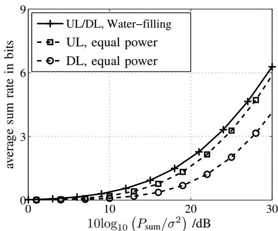
Fig. 5. Average sum rate per transmission phase based on interference leakage minimization solutions
