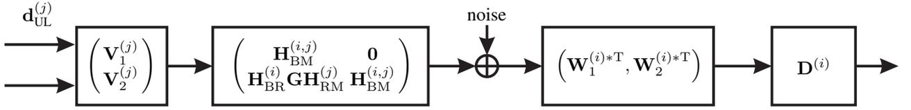
Fig. 2. Equivalent block diagram of the UL transmission from the MSs in the  $j$ -th cell to the  $i$ -th BS
