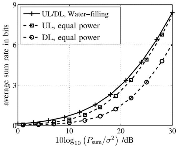
Fig. 4. Average sum rate per transmission phase based on linear IA solutions
