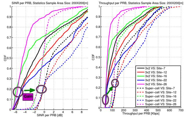
Fig. 4. SINR per PRB and Throughput per PRB performance Comparison for a 3x2 and Super-cell VS for selected sites.
