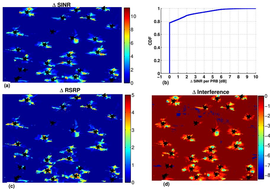
Fig. 3. Observed change in SINR, RSRP and Interference after a super-cell configuration is employed in AAS-based 3x2 VS [colorbar scale in dB].
