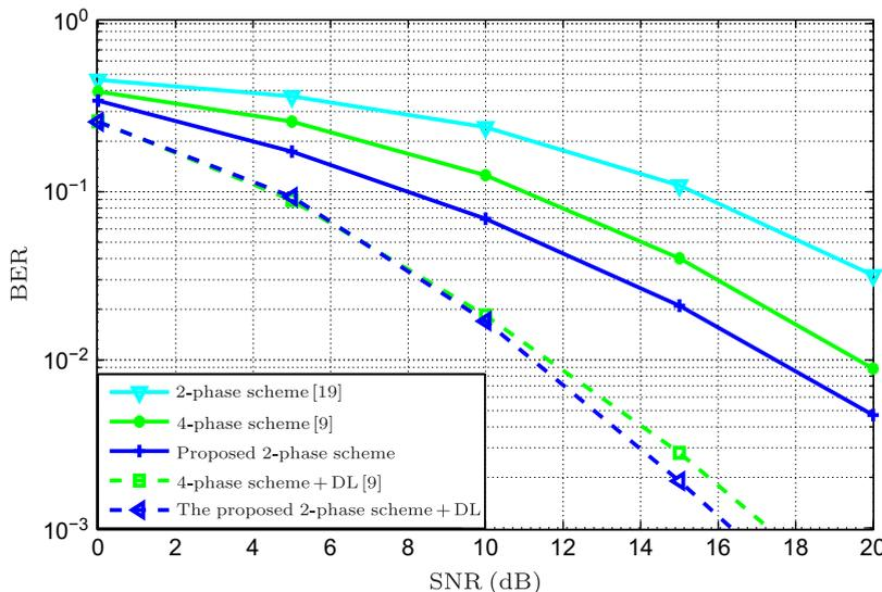
Fig. 6. BER versus SNR for several differential schemes with  $R=2$  and a rate of 0.5 bpcu.
