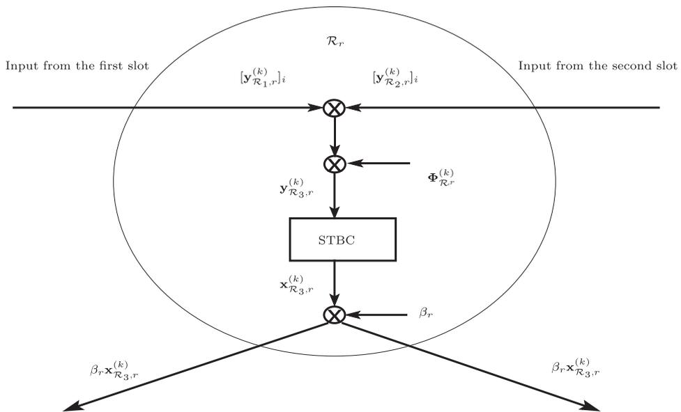
Fig. 4. Combination procedure at the rth relay.
