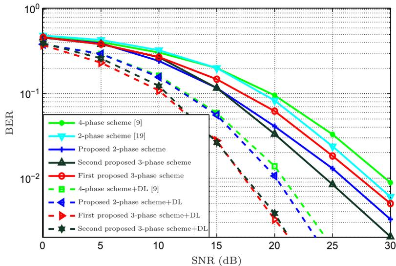
Fig. 7. BER versus SNR for several differential schemes with  $R=2$  and a rate of 1 bpcu.
