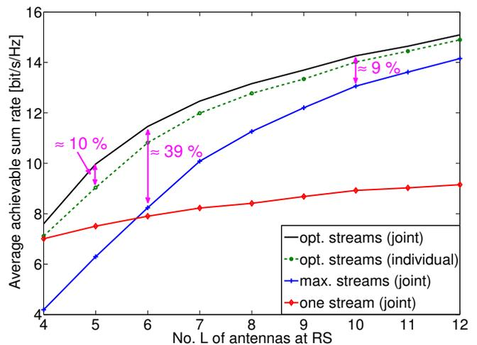
Fig. 3. Average achievable sum rates over number  $L$  of antennas at RS for  $\mathbf{r} = (1, 0.5, 0.5, 0.25)$ ,  $M = 2$ ,  $K = 2$ , average receive SNR at RS = 15dB.
