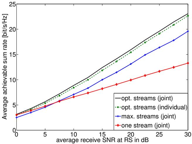
Fig. 4. Average achievable sum rates over different receive SNRs at RS for  $\mathbf{r} = (1, 0.5, 0.5, 0.25)$ ,  $M = 2$ ,  $K = 2$ ,  $L = 7$ .
