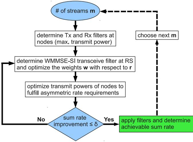
Fig. 2. Considered subproblems for maximizing the achievable sum rate under asymmetric rate requirements.
