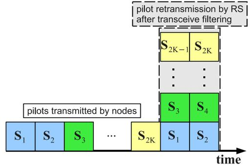
Fig. 2. Pilot transmission scheme for multi-pair two-way relaying.
