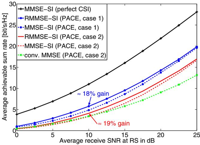
Fig. 3. Average achievable sum rates versus average receive SNR at RS for  $L = 8$  considering one transmitted pilot symbol per node.
