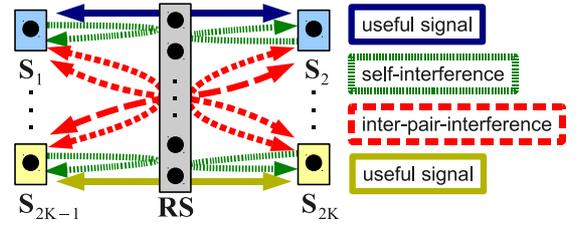
Fig. 1. Composition of useful signals and interferences in a bidirectional multi-pair two-way relaying scenario.
