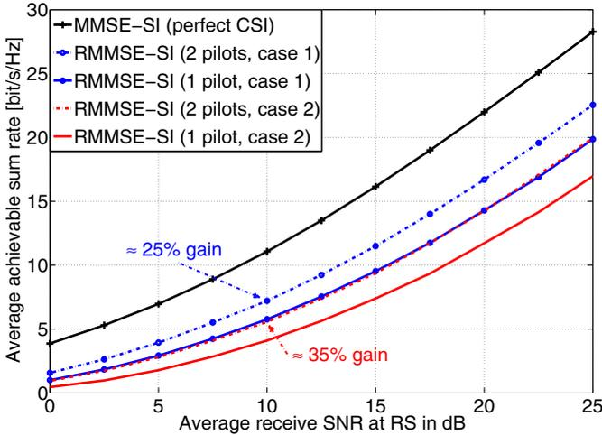
Fig. 4. Average achievable sum rates versus average receive SNR at RS for  $L = 8$  considering one and two transmitted pilot symbols per node.
