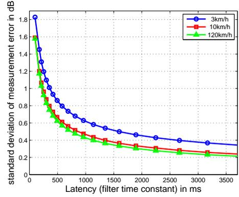
Fig. 1. Trade-off between latency and measurement error  $\mathbf{e}_{u,c}(t)$
