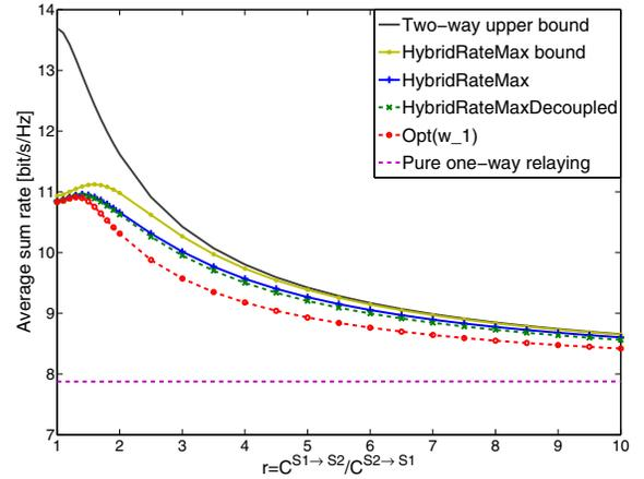
Fig. 3. Average sum rates for different rate constraints,  $M = 4$ ,  $L = 6$ ,  $\text{SNR}_1 = \text{SNR}_2 = 15\text{dB}$ .
