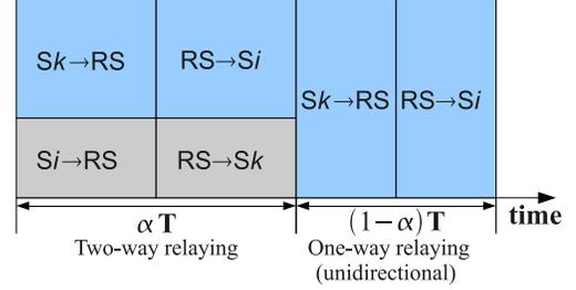
Fig. 2. Hybrid one-way / two-way relaying scheme.
