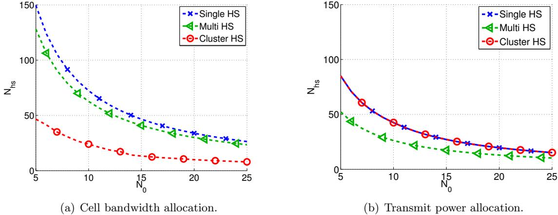
Figure 2: Maximum number  $N_{\text{hs}}$  of users in a hotspot cell in dependence of the number  $N_0$  of users in the remaining cells for 5 % cell outage probability.
