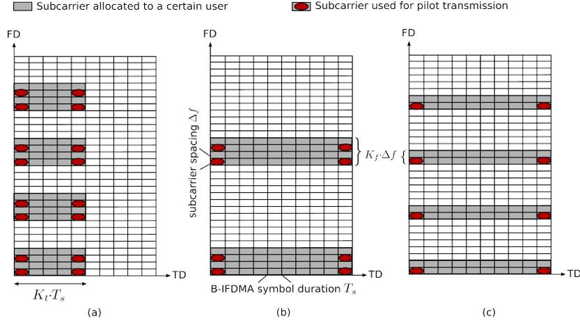
Figure 1. Exemplary subcarrier allocations and pilot arrangements for B-IFDMA (a)  $K_t = 5$ ,  $Q = 16$ ,  $K_f = 4$  (b)  $K_t = 10$ ,  $Q = 8$ ,  $K_f = 4$ , (c)  $K_t = 10$ ,  $Q = 8$ ,  $K_f = 2$ .
