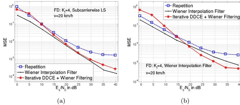
Figure 2. Comparison of Repetition, Wiener Interpolation Filter and iterative DDCE + Wiener Filtering in TD for (a) Subcarrierwise LS estimation in FD and  $v = 20$  km/h, (b) Wiener Interpolation Filter in FD and  $v = 20$  km/h.
