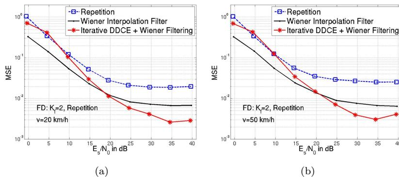
Figure 3. Comparison of Repetition, Wiener Interpolation Filter and iterative DDCE + Wiener Filtering in TD for (a) interpolation with Repetition in FD for  $v = 20$  km/h, (c) interpolation with Repetition in FD for  $v = 50$  km/h .
