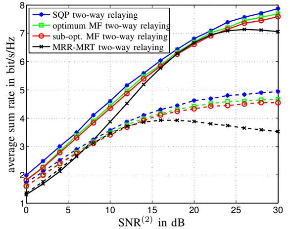
Figure 1. Average sum rate for different approaches in CASE1 and CASE3,  $M = 1$ ,  $L = 4$  (dashed lines:  $\text{SNR}^{(1)} = 10\text{dB}$ , solid lines:  $\text{SNR}^{(1)} = 20\text{dB}$ )
