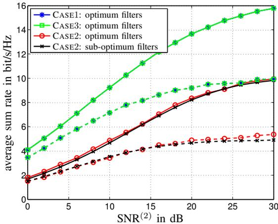
Figure 2. Average sum rate for all optimum cases; average sum rate for sub-optimum CASE2,  $M = 2$ ,  $L = 8$  (dashed lines:  $\text{SNR}^{(1)} = 10\text{dB}$ , solid lines:  $\text{SNR}^{(1)} = 20\text{dB}$ )
