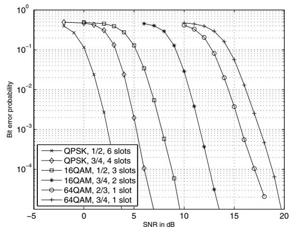
Figure 1: Bit error probability for AWGN channel.
