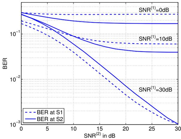
Fig. 4. Comparison of BER performance at  $S1$  and  $S2$  for the linear MMSE transceiver filter for different fixed values of  $SNR^{(1)}$
