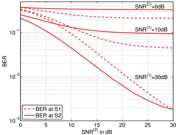
Fig. 3. Comparison of BER performance at  $S1$  and  $S2$  for the linear ZF transceiver filter for different fixed values of  $SNR^{(1)}$
