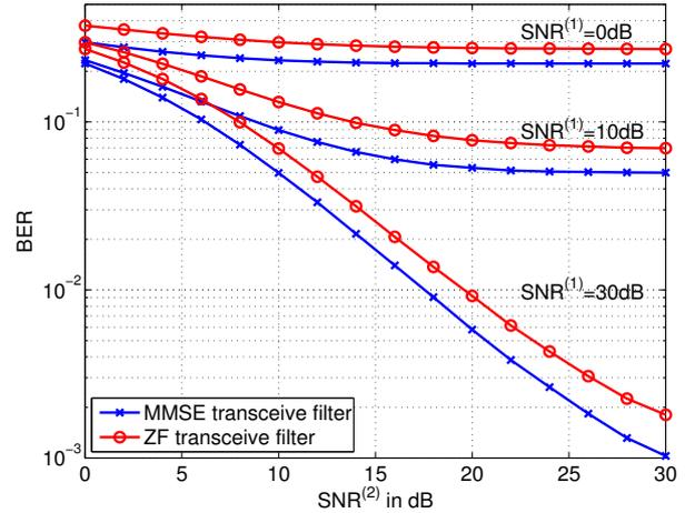
Fig. 2. Comparison of overall BER performance at  $S2$  for the linear ZF and MMSE transceive filter for different fixed values of  $\text{SNR}^{(1)}$
