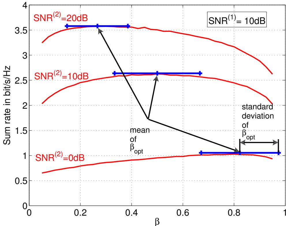
Figure 3: Sum rate depending on  $\beta$  with fixed  $\text{SNR}^{(1)} = 10\text{dB}$  and  $\text{SNR}^{(2)}$  as a parameter
