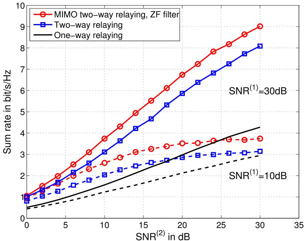
Figure 2: Sum rate of different relaying protocols depending on  $\text{SNR}^{(2)}$  with  $\text{SNR}^{(1)}$  as a parameter;  $\beta = 0.5$  for MIMO two-way relaying; dashed lines:  $\text{SNR}^{(1)} = 10\text{dB}$ , solid lines:  $\text{SNR}^{(1)} = 30\text{dB}$
