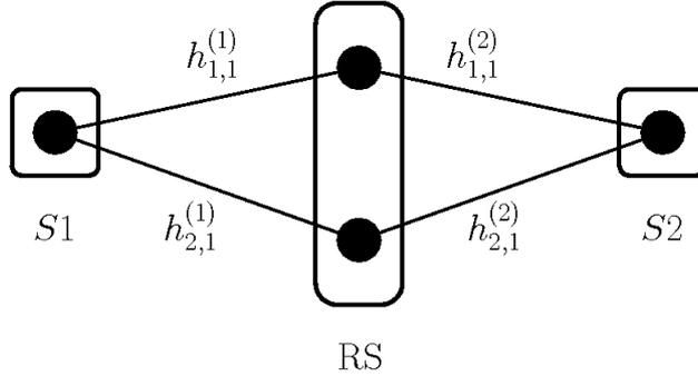
Figure 1: Relay network for  $M^{(1)} = 1$  antenna at  $S1$ ,  $M^{(2)} = 1$  antenna at  $S2$ , and  $M_{\text{RS}} = 2$  antennas at the RS
