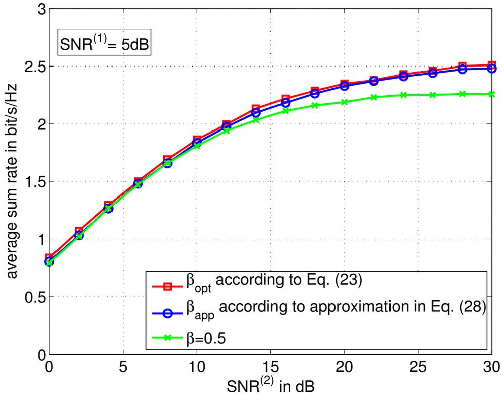
Figure 4: Average sum capacity depending on  $\text{SNR}^{(2)}$  for fixed  $\text{SNR}^{(1)} = 5\text{dB}$ : comparison of results from Eq. (23), Eq. (28), and  $\beta = 0.5$
