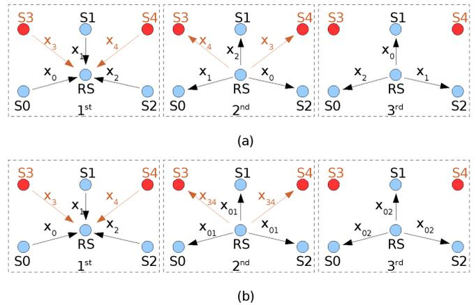
Fig. 1. Multi-group multi-way relaying: (a). Without analog network coding (ANC); (b). With ANC.
