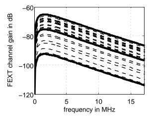
Fig. 2: 24 FEXT channels of victim line  $n_V$ . The channels of disturbers  $n_A$ ,  $n_B$  and  $n_C$  are drawn with solid lines.
