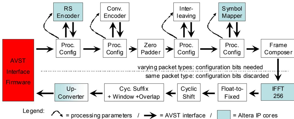
**Figure 9: Block diagram of transmitter signal generation architecture.**
