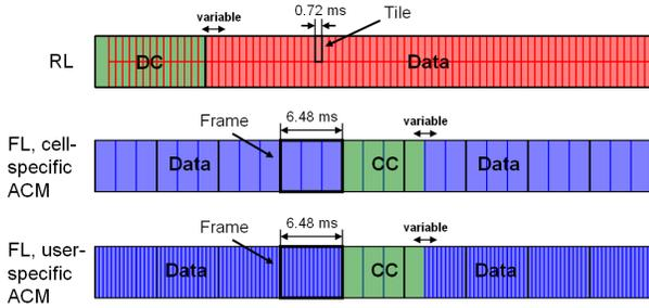
**Figure 6: Multi-Frame structure.**
