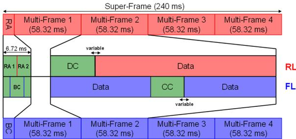
**Figure 5: Super-Frame structure.**
