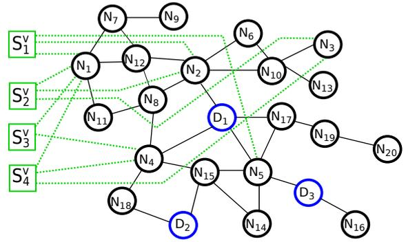
Figure 2: For the four parts  $F_1$ ,  $F_2$ ,  $F_3$  and  $F_4$  of content  $F$ , four virtual sources  $S_1^v$ ,  $S_2^v$ ,  $S_3^v$  and  $S_4^v$  are introduced, which are connected via virtual links with nodes that have the respective part in their cache, indicated by green dotted lines.
