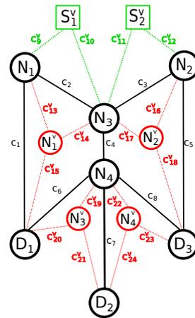
Figure 3: Virtual sources  $S_1^v$  and  $S_2^v$  represent parts  $F_1$  and  $F_2$  of content  $F$  and are connected through virtual links to nodes which have cached  $F_1$  or  $F_2$ , respectively. Virtual nodes  $N_1^v$  and  $N_2^v$  represent the broadcast of  $N_1$  and  $N_2$ , respectively, while  $N_3^v$  and  $N_4^v$  represent two possible multicasts of  $N_4$ .
