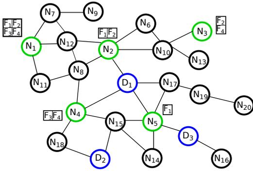
Figure 1: Destinations  $D_1$ ,  $D_2$  and  $D_3$ , marked in blue, request content  $F$ , which is distributed over the wireless multihop network, where nodes with the complete or part of the content in the cache are marked in green.
