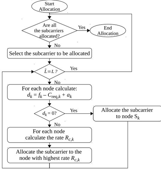
Fig. 2. Flow diagram of the resource allocation algorithm
