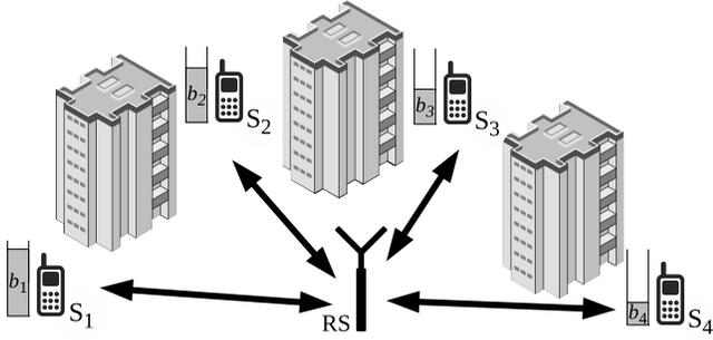
Fig. 1. Multi-way relaying scenario consisting of  $K = 4$  single-antenna nodes with different buffer levels and a multi-antenna relay station, termed RS.
