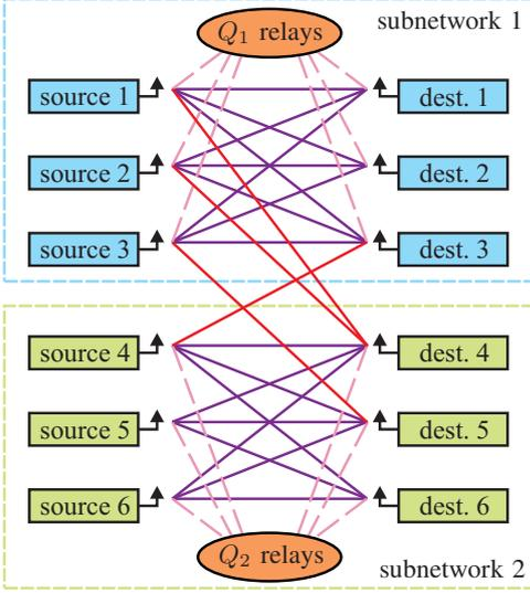
Fig. 1. A network made up of two partially connected subnetworks with  $Q_1$  and  $Q_2$  single-antenna relays, respectively
