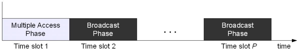
Figure 3.2. Communication protocol for MGMW relaying
