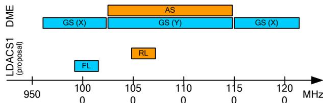
**Figure 8. Frequency Allocation of DME and LDACS1**
