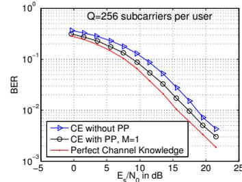
Fig. 1. Uncoded BER performance for CE with and without PP
